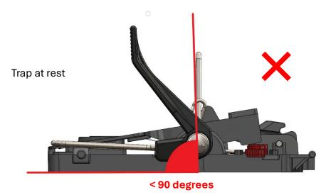
The strike bar is 90 degrees or less to trap base as shown
